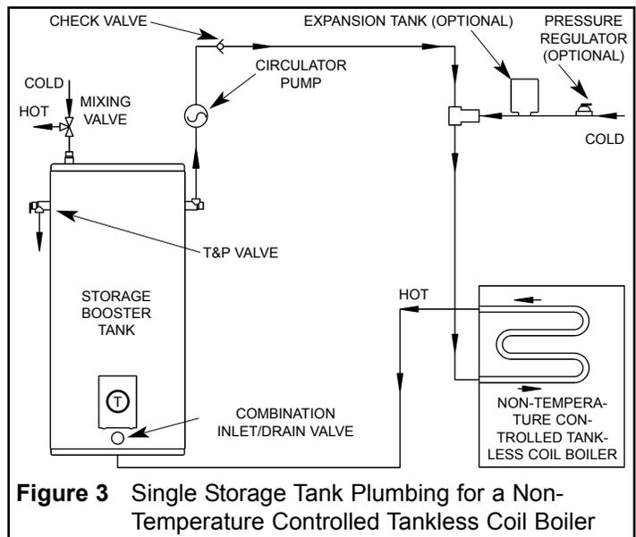
**Figure 3** Single Storage Tank Plumbing for a Non-Temperature Controlled Tankless Coil Boiler
