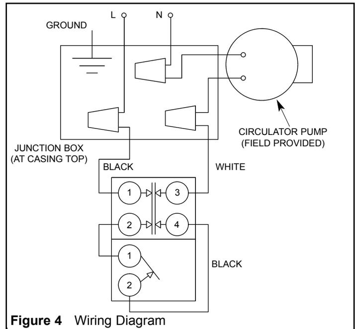
**Figure 4** Wiring Diagram
