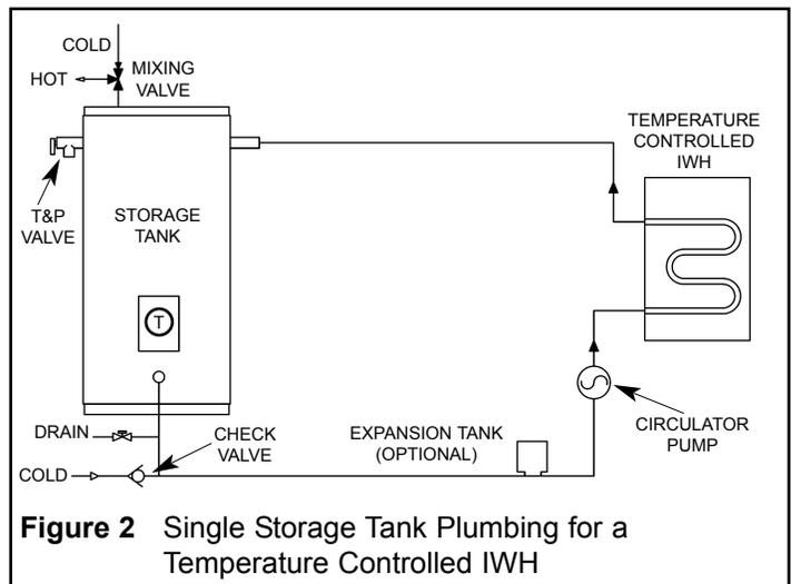
**Figure 2** Single Storage Tank Plumbing for a Temperature Controlled IWH
