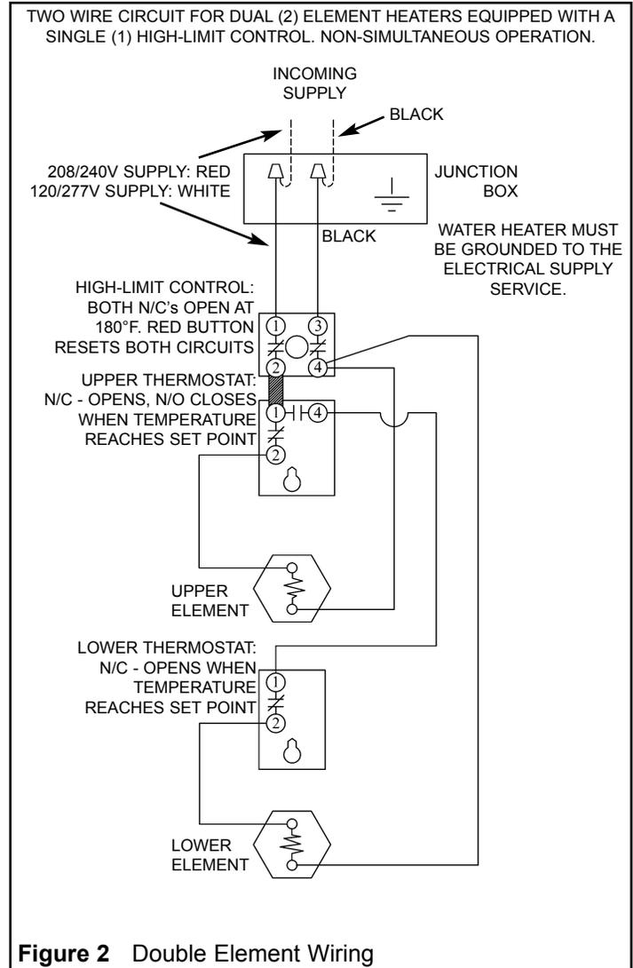
**Normal Operation:** When hot water is being used, cold water enters the bottom of the heater (either bottom feed or by diptube), and the bottom element will begin to heat the cold water. If lots of hot water has been used, the upper thermostat will take priority and the top portion of the heater will be heated. Once heated, the thermostat will flip down to the lower thermostat to heat the lower portion.
