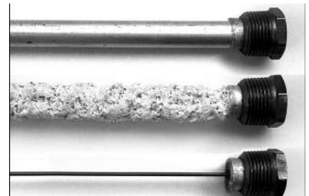
Figure 27 - Anode Rods from new (top) to partially depleted (middle) to fully depleted stage (bottom)
