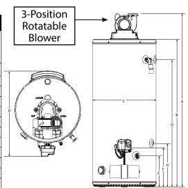
For propane models sub N with P. Natural gas models are series 200/300. Propane models are series 201/301. All models comply with national energy efficiency regulations.
